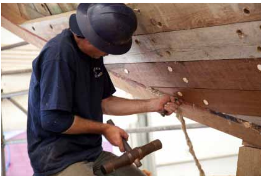
More than five miles of cotton and oakum were used between the planks of the Bluenose II hull. Photo by Mark Doucette.
